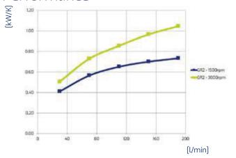
Oil T 80°C T Amb. 40°C  $1 \, \text{kW} = 860 \, \text{Kcal/h} - 1 \, \text{HP} = 0.75 \, \text{kW}$
