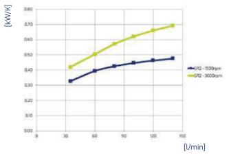
Oil T 80°C T Amb. 40°C 1 kW = 860 Kcal/h – 1 HP = 0,75 kW
