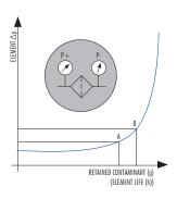
The **Pressure Drop** (Dp = differential pressure) through the filter increases during the system operation due to the contaminant retained by the filter element.
