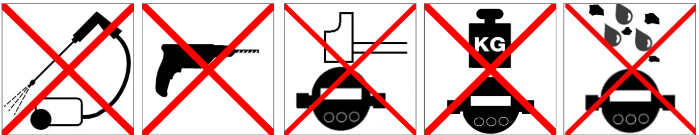
Fig. 9: Inadmissible mechanical stress
