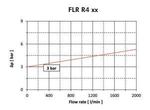
N.B. All the reported data have been obtained at our laboratory, according to specification ISO3968 with mineral oil having 32 cSt viscosity and density 0,875 Kg/dm<sup>3</sup>.
