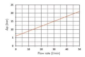
N.B. All the reported data have been obtained at our laboratory, according to specification ISO3968 with mineral oil having 32 cSt viscosity and density 0,875 Kg/dm³.
