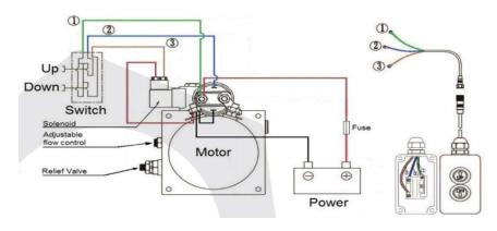
A minimum of 25mm2 cable at a max length of 5 metres is recommended with the negative cable in one continuous length from the battery terminating at the power unit. A 210amp fuse should be used if operating at full load.
