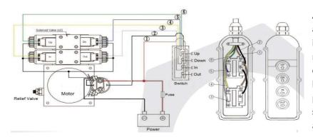
A minimum of 25mm2 cable at a max length of 5 metres is recommended with the negative cable in one continuous length from the battery terminating at the power unit. A 210amp fuse should be used if operating at full load.
