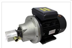
This two stage motor pump set can offer a faster cycle time than a conventional gear motor setup. The Hi-Lo Pump is preset at 900 psi for the low pressure pump and 3000 psi for the high pressure. The change from Lo to Hi pressure is automatic with the Lo side pressure pre set from 400 psi to 900 psi.
