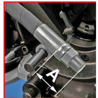
The dimension from the face of the fitting to the crimp position will now be the dimension established in the previous step.
