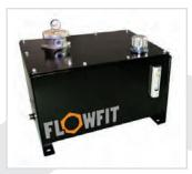
100 Litre capacity tank kits supplied with tank, return line filter, level indicator, filler breather and drain plug along with all required nuts and bolts. All components are supplied loose and ready to assemble with all necessary holes pre-drilled on tank. Comes painted in black but available in grey primer if required.
