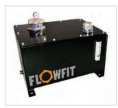
14 Litre capacity tank kits supplied with tank,return line filter, level indicator, filler breather and drain plug along with all required nuts and bolts. All components are supplied loose and ready to assemble with all necessary holes pre-drilled on tank. Comes painted in black but available in grey primer if required.
