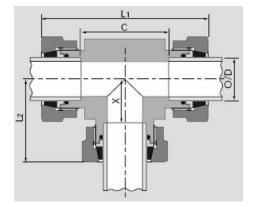
Working Temperature: Nitrile: -40°C to +100°C Viton: -20°C to +150°C
