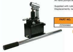
Supplied with rubber protection for the piston, pressure relief valve and 4/3 flow divider closed centre. Displacements, tank size and pressures as shown in the table below.
