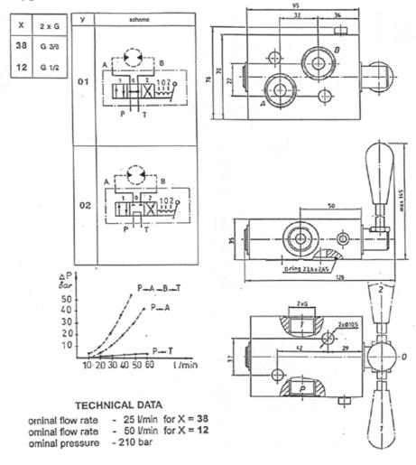
Manifold Mounts Directly onto ports of EPMS (OMS) motor
