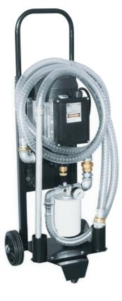
The HF10 range of trollies is the ideal tool for decontaminating oil by removing suspended particles either by flushing or continuous cleaning. It is well suited for prefiltering and transfer of fluids as well as removing water from hydraulic systems (Optional water removal filter required)
