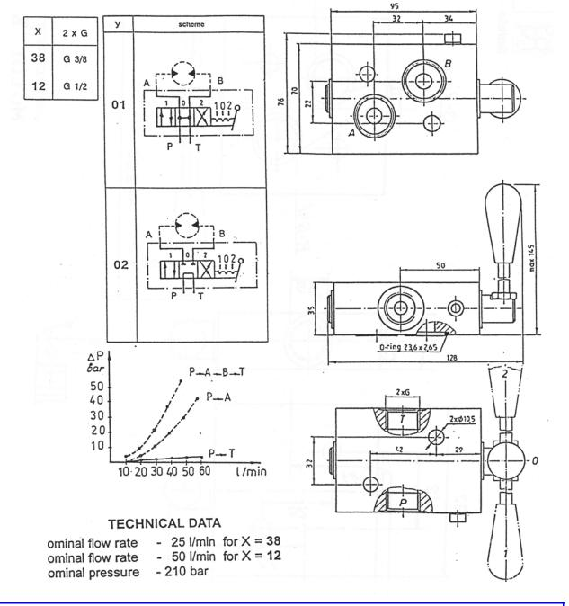
Manifold Mounts Directly onto ports of EPMS (OMS) motor
