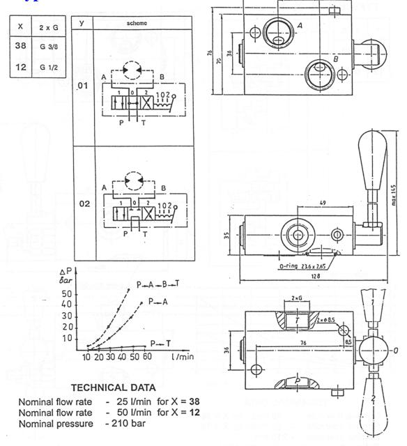
Manifold Mounts Directly onto ports of EPM & EPRM (OMP & OMR) motor
