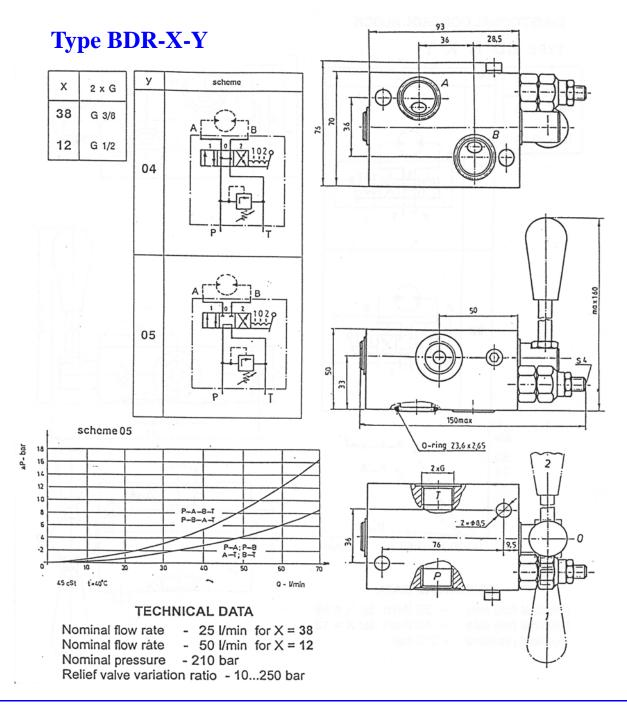
Manifold Mounts Directly onto ports of EPM & EPRM (OMP & OMR) motor
