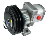
MOUNTED INLINE ENGINE BELT 2 GOOVE PULLEY, CLOCKWISE ROTATION-MAX 3000RPM, AVAILIBLE ELECTRICIAL 12V INPUT AT 3A NOMINAL TORQUE, FLOW RATES AND VOLTAGES SHOWN IN FULL BELOW.
