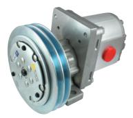
MOUNTED INLINE ENGINE BELT 2 GOOVE PULLEY, CLOCKWISE ROTATION-MAX 3000RPM, AVAILIBLE ELECTRICIAL 12V INPUT AT 5A NOMINAL TORQUE, FLOW RATES AND VOLTAGES SHOWN IN FULL BELOW.
