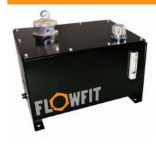
58 Litre capacity tank kits supplied with tank,return line filter, level indicator, filler breather and drain plug along with all required nuts and bolts. All components are supplied loose and ready to assemble with all necessary holes pre-drilled on tank. Comes painted in black but available in grey primer if required.
