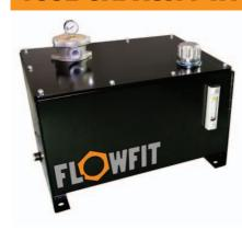
165 Litre capacity tank kits supplied with tank, return line filter, level indicator, filler breather and drain plug along with all required nuts and bolts. All components are supplied loose and ready to assemble with all necessary holes pre-drilled on tank. Comes painted in black but available in grey primer if required.
