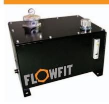
100 Litre capacity tank kits supplied with tank, return line filter, level indicator, filler breather and drain plug along with all required nuts and bolts. All components are supplied loose and ready to assemble with all necessary holes pre-drilled on tank. Comes painted in black but available in grey primer if required.
