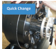
Easy positioning of fitting thanks to radial die movement
