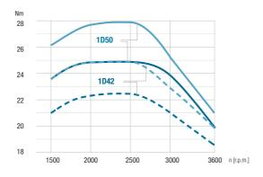
▶ Performance data refer to Standard Reference Conditions of ISO 3046-1: + 25 °C (77 °F), 100 kPa, relative humidity 30 %. During running-in period the output increases by approx. 5 % which is taken into consideration at delivery. Power reduction acc. to ISO 3046-1. Standard values:
