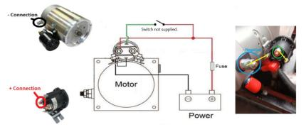
A minimum of 25mm2 cable at a max length of 5 metres is recommended with the negative cable in one continuous length from the battery terminating at the power unit. A 210amp fuse should be used if operating at full load.
