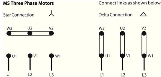
1ph motors are wired differently to 3ph motors and rotation is changed by different positions of the linking bars and supply cables. The wiring for different rotations is as below:
