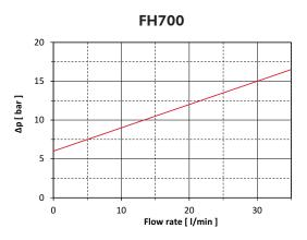
N.B. All the reported data have been obtained at our laboratory, according to specification ISO3968 with mineral oil having 32 cSt viscosity and density 0,875 Kg/dm<sup>3</sup>.
