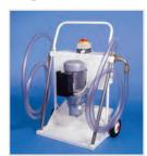
The super deluxe portable filtration unit offers flow rates upto 75 l/min with filtration levels available from 3 micron upto 25 micron on return and 25 micron upto 125 micron on suction.
