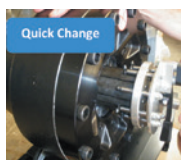
Easy positioning of fitting thanks to radial die movement
