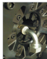
Front flange cuts allow long drop elbows
