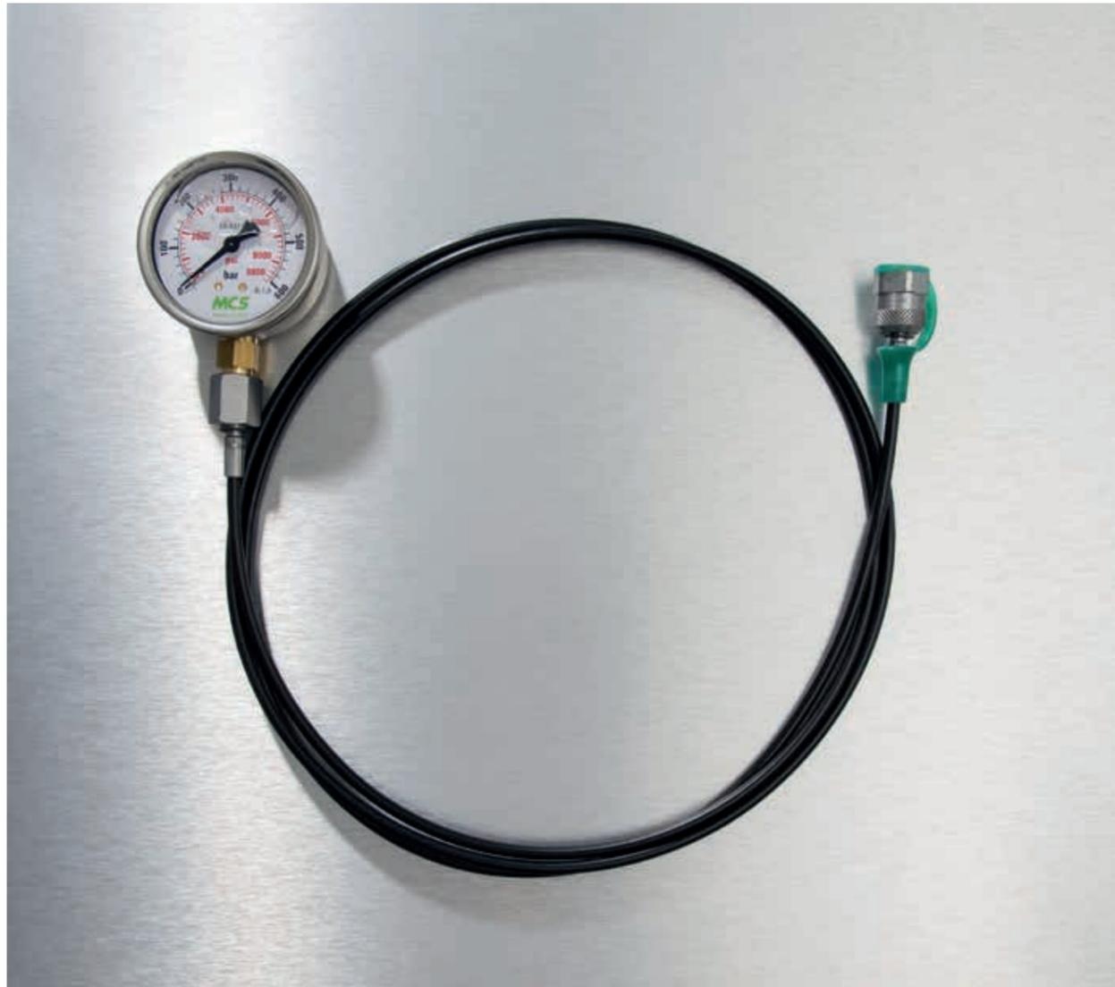
Hoses and fittings, pressure can be checked while hydraulic systems are at full pressure. Micro-fittings and micro-bore hoses can bear a working pressure of max. 630 bar.
